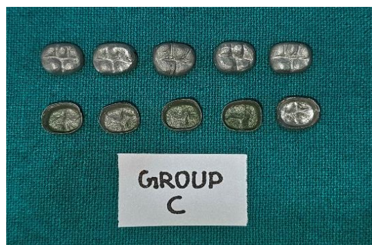
Figure 3: Metal Copings fabricated by DMLS (n=10)
