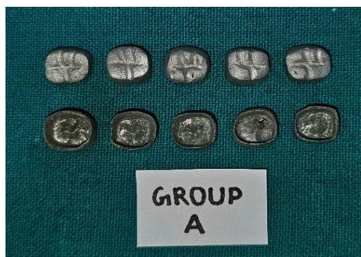
Figure 1: Metal copings fabricated by casting (n=10)
