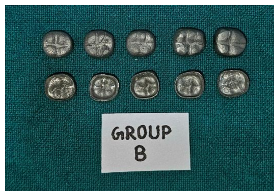
Figure 2: Metal copings fabricated by CAD/CAM (n=10)
